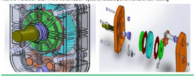
Reliable performance of self-locking, accurate limit range, automatic brake holds sidewall in place
