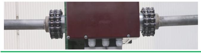
3GG Gear Motor: the self-braking performance is excellent and meets the standards of a high precision window opening system
